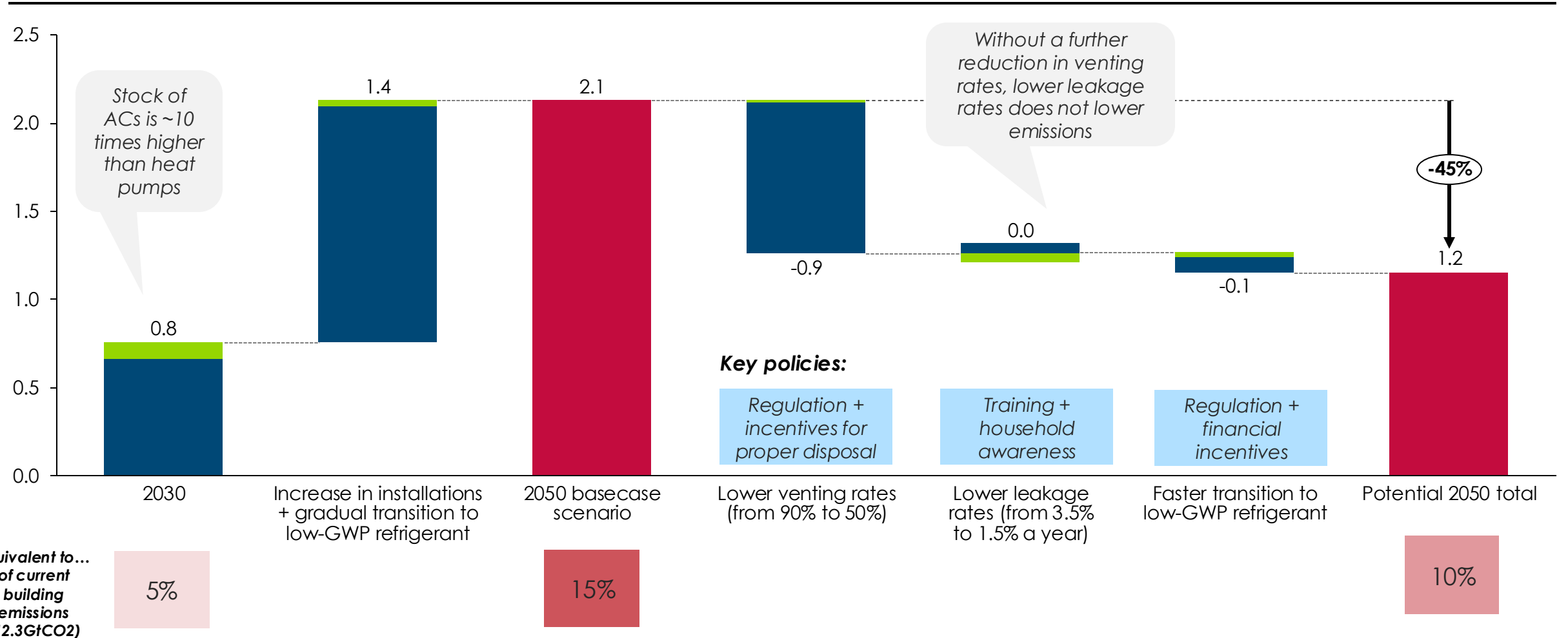
Scenarios of potential annual global emissions relating to refrigerant leakage and venting
